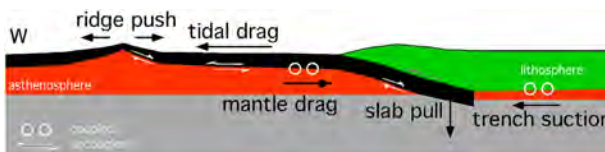
Figure 69 Main system of forces that may act on the lithosphere. Mantle drag and trench suction need high coupling (relatively higher viscosity) between lithosphere and asthenosphere to be effective. Ridge push, slab pull, and tidal drag rather need low coupling (relatively lower viscosity) to be efficient. Since the lithosphere is decoupled with respect to the asthenosphere, more than one force is acting on plate motions. Circles indicate coupled forces while white half arrows show the uncoupled forces. After Doglionni et al. (2007) .
