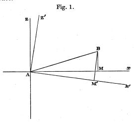
zontal distance between A and B, and AM' the calculated horizontal distance. Hence the calculation makes this portion of the arc too short by
