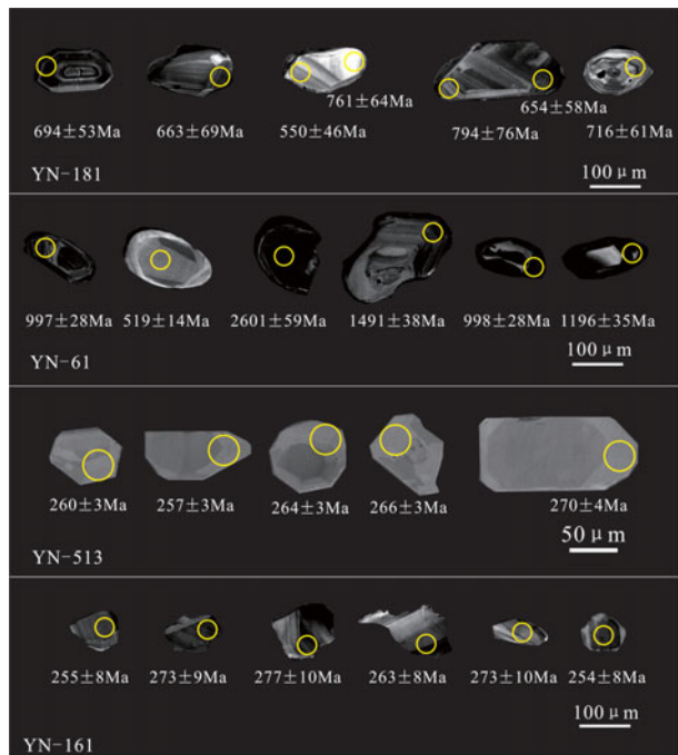
Figure 7. (Colour online) Representative CL images of analysed zircons from sandstone samples YN-61, YN-161, YN-181 and YN-513, collected from Binchuan, Xichang, Ertan and Muli, respectively. Analysis spots are indicated by yellow circles, and calculated ^{206}\text{Pb}/^{238}\text{U} ages are indicated. Other CL images are shown in Data Repository 1 (in Supplementary Material at https://doi.org/10.1017/S0016756818000171 ).
