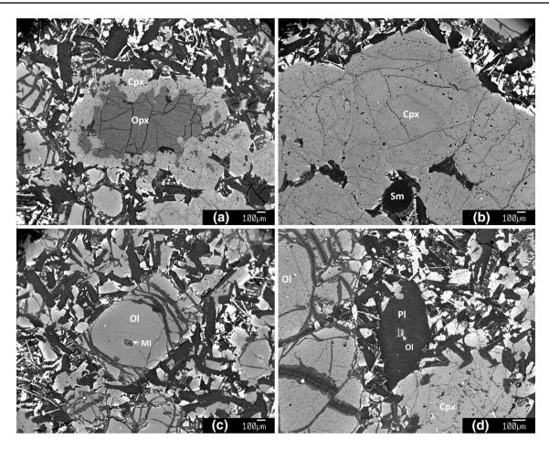
**Fig. 4** a Augitic clinopyroxene (Cpx) overgrowth on orthopyroxene (Opx). **b** Oscillatory-zoned Cpx with glass inclusion altered to smectitic clay (sm). **c** Olivine (Ol) with alteration veins and melt inclusion
